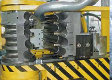
Achieving the optimum wall-thickness, bend radiuses and folding characteristics pose problems for many users. The solution: Special bending media.
