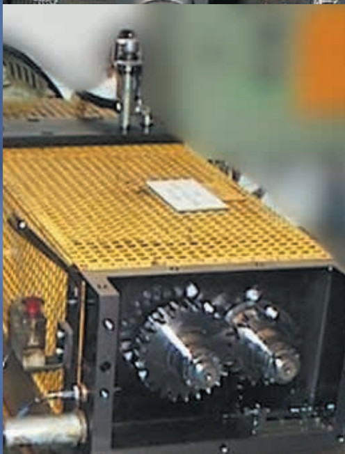
FZG Gear test rig to test the load carrying capacity of EP/AW gear oils and lubricating oils
