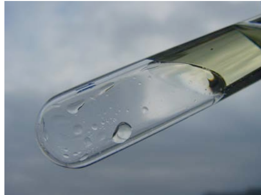
Fig. 7: 2-phase system refrigerant R422D (colourless) – mineral oil-based refrigeration oil RENISO KM 32 (yellowish)
